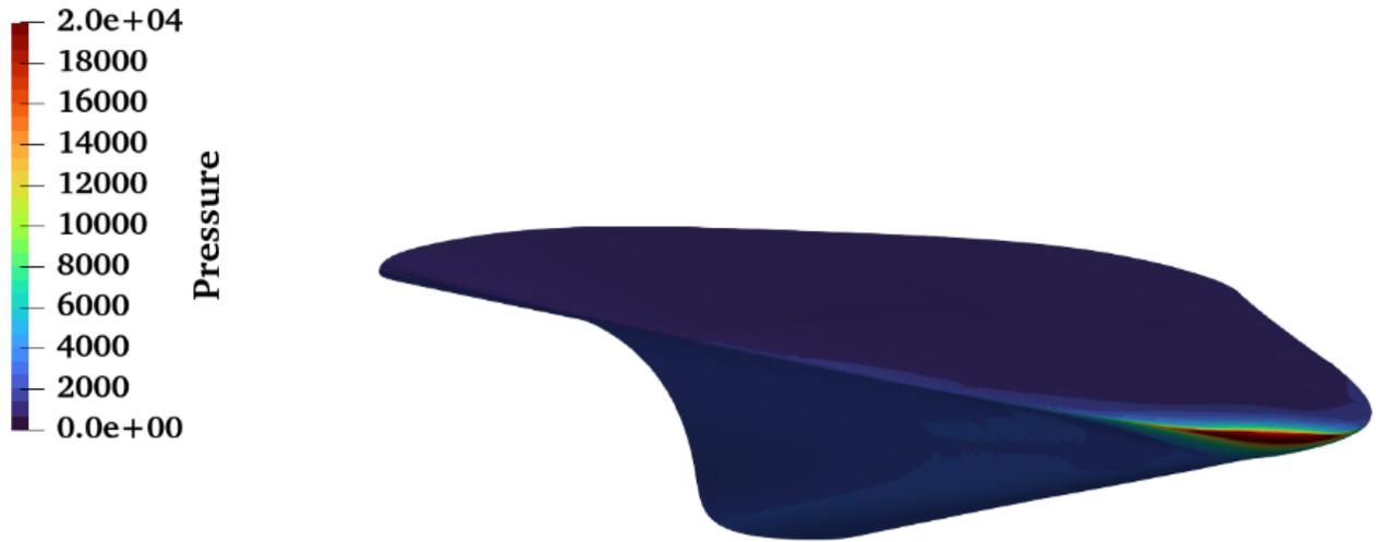
*Figure 87: Pressure contours on the vehicle's surface.*
