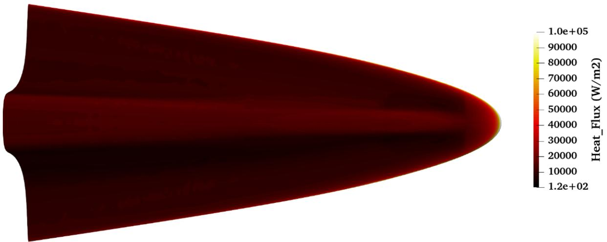
**Figure 75:** Heat flux at the bottom surface of the vehicle (0.0 AoA) (Scale reduced for better visualization. Maximum value 250,000 W/m<sup>2</sup>).
