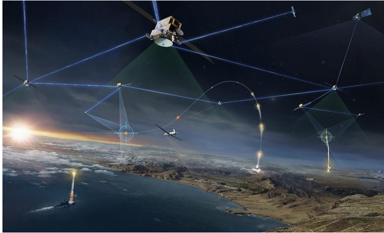
Northrop Grumman's proposed Tranche 1 Transport Layer (T1TL) mesh satellite communications network, a constellation of 42 low-Earth orbit satellites, aims to provide resilient, low-latency, high-volume data transport.
